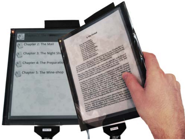
Figure 4. Pointing with a hot display (right) into a warm display, in this case showing a TOC (left), displays detailed focus information on the hot display, in this case a book page.
