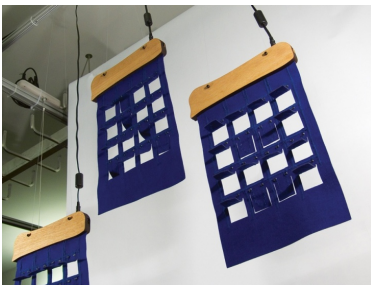
figure 4. Shape changing textile surface for environmental control and communication [1].
