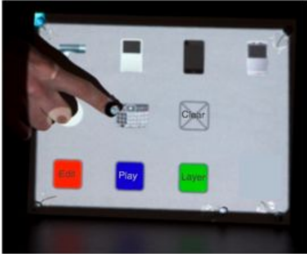
Figure 5. Interaction Palette showing interaction elements on a piece of cardboard with IR reflective markers.
