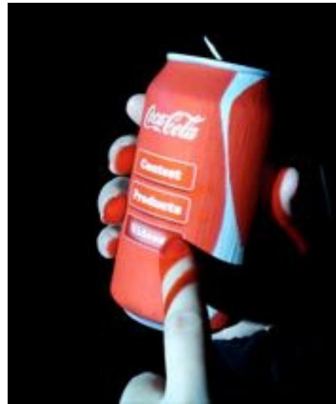
Figure 7. Five cent interactive beverage can prototype. Please note that Vicon markers appear on the back.
